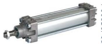
The <u>RA/8000 Series Norgren pneumatic actuator</u> is a double acting cylinder, with a tie-rod design. This cylinder conforms to ISO/VDMA standards and can be specially manufactured to perform well in ATEX areas. Offering high performance, this component is a reliable pneumatic cylinder for applications that require double acting control. The wide bore sizes and long stroke lengths make this ATEX pneumatic cylinder a versatile, high functioning solution.
