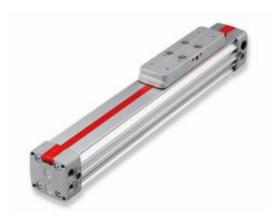
The Lintra® Plus Series are high-performance units that have been designed to deliver reliable and optimum performance in a wide range of process industry applications. Available in sizes from 16mm – 80mm bore and with strokes of up to 8500mm, they have a lightweight design and are fitted with dust protection as standard.
