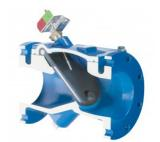
Weight and lever swing non return check valves are available in a wide range of materials, including, cast iron, ductile iron and stainless steel. Swing type nrvs are available with optional springs, weight, levers and guards.
