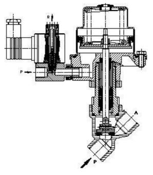
When pressure is connected to port "Z" the valves open or close according to type. A separate 3/2 pilot valve is used to supply pressure to port "Z", it is mounted either directly on the actuator or remotely.
