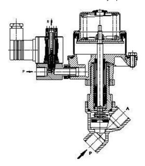
When the pilot valve is de-energised the supply pressure is shut off and the air pressure within the chamber vents to atmosphere. The piston/diaphragm now returns under spring pressure, the valve seal covers the valve seat and the valve closes and remains closed under spring pressure. In some versions (closing with the flow) the fluid exerts a pressure on top of the valve seal that assists the closing process.
