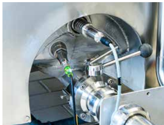
The hygienic pressure sensor PBMN Flush and the level switch CleverLevel LBFS monitor the level in the mixing tanks. Thanks to the precise sensors, downtimes could be minimized considerably.
